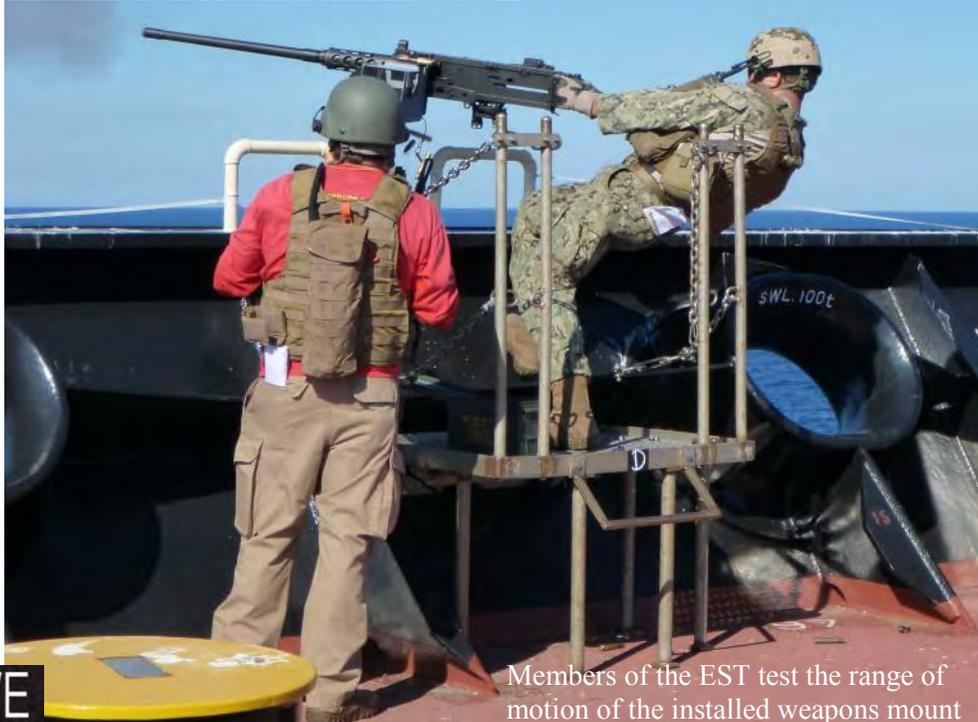
Members of the EST test the range of motion of the installed weapons mount
