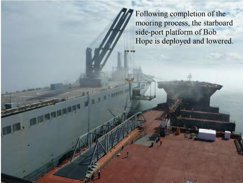
Following completion of the mooring process, the starboard side-port platform of Bob Hope is deployed and lowered.
