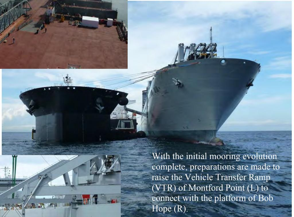
With the initial mooring evolution complete, preparations are made to raise the Vehicle Transfer Ramp (VTR) of Montford Point (L) to connect with the platform of Bob Hope (R).
