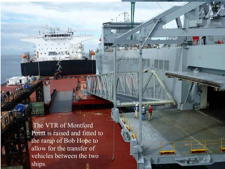
The VTR of Montford Point is raised and fitted to the ramp of Bob Hope to allow for the transfer of vehicles between the two ships.
